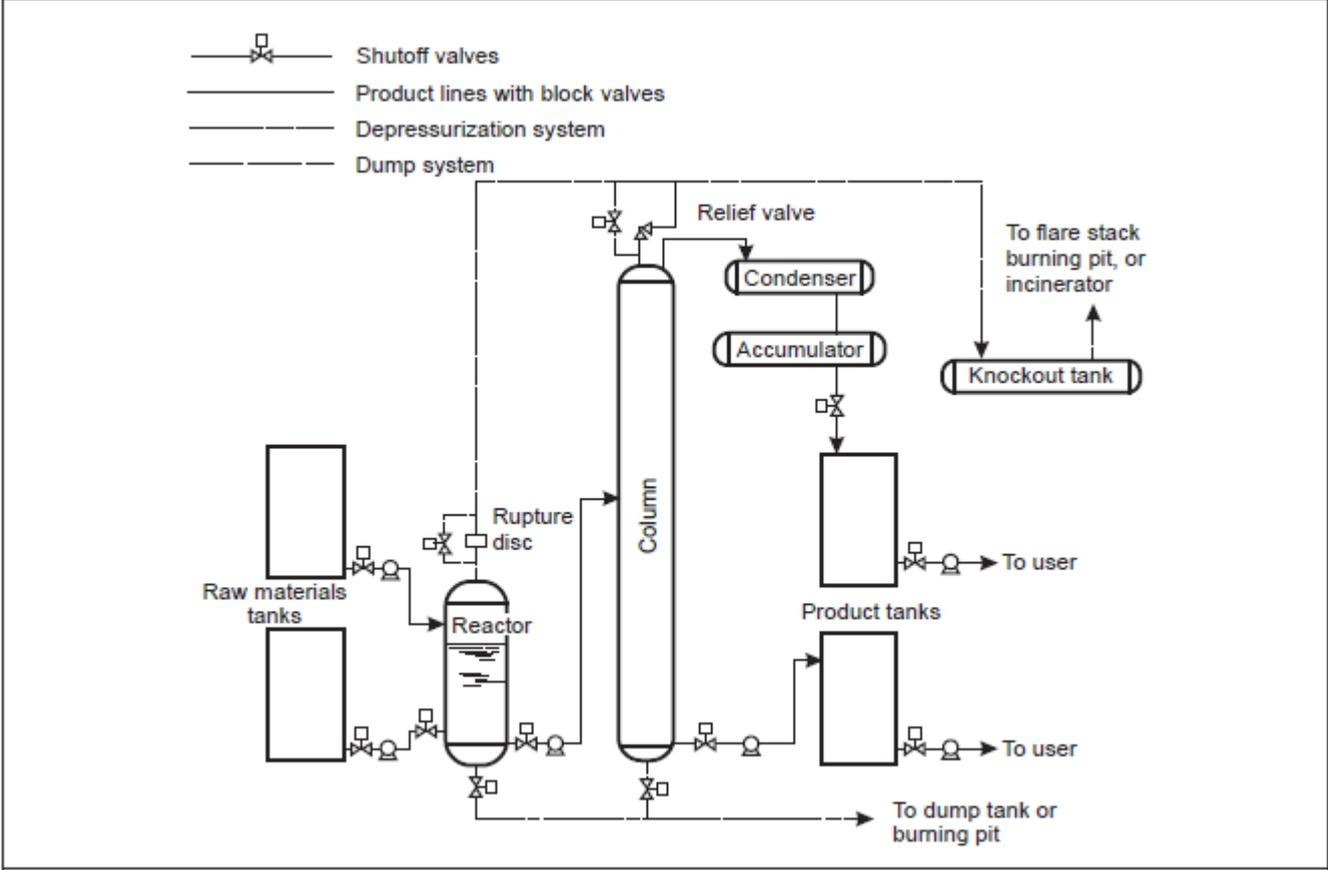
Fig. 10. Accidental release control systems and valves
